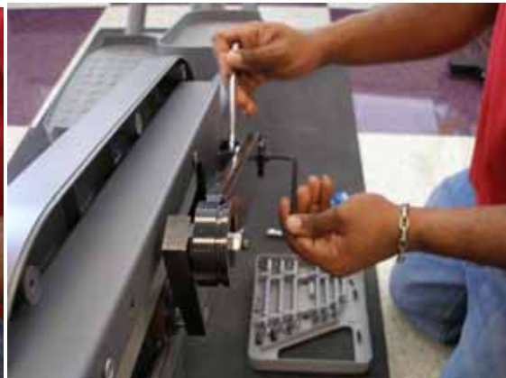
Fig. 8: installing the new control link assembly
